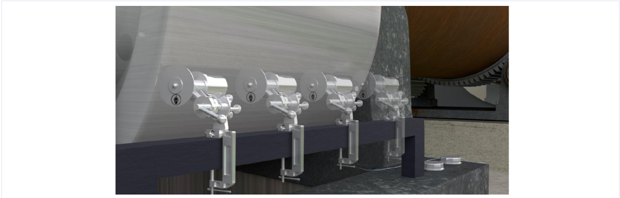
Example of measuring wheel placement at different positions across the width for diameter and cylindricity review.
